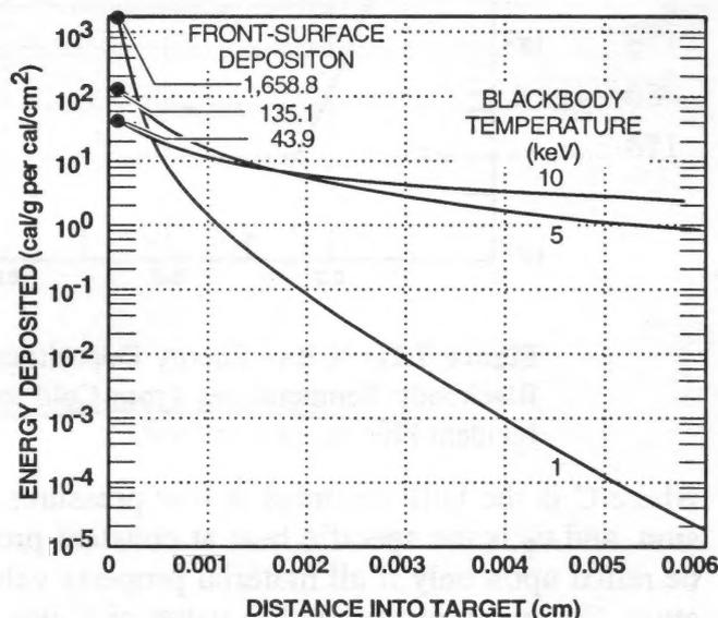
Figure 7.10. ANISN Deposition Profile for Tantalum at Blackbody Temperatures of 1, 5, and 10 keV (Incident Fluence = 1 cal/cm<sup>2</sup>).
